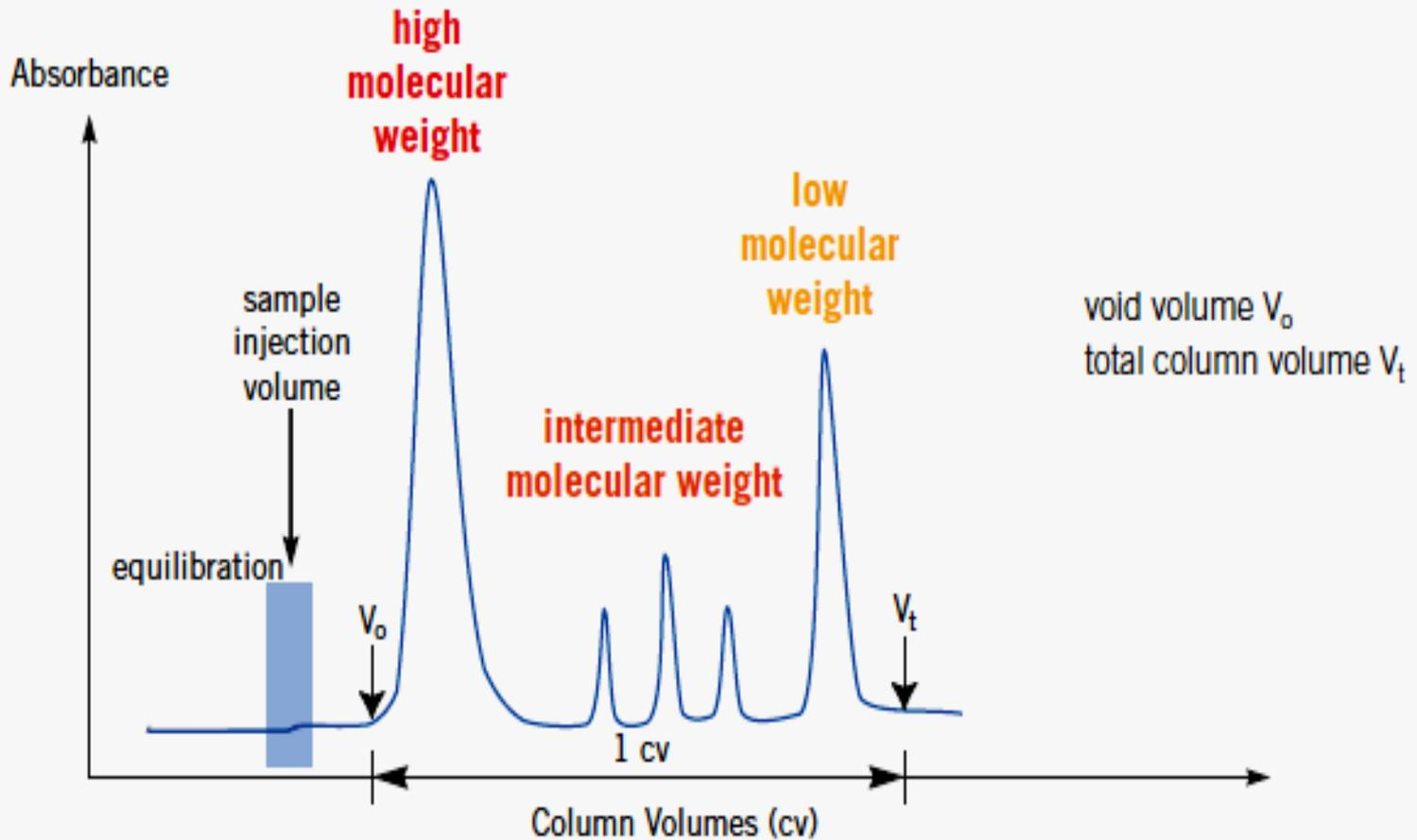
**Theoretical chromatogram of a high resolution fractionation (UV absorbance detector of biomacromolecules)**
